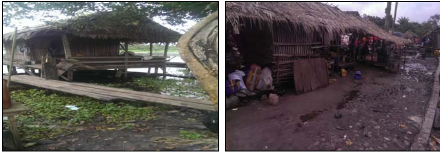
Figure 2. Building built with raffia palm pole in the Study Area
